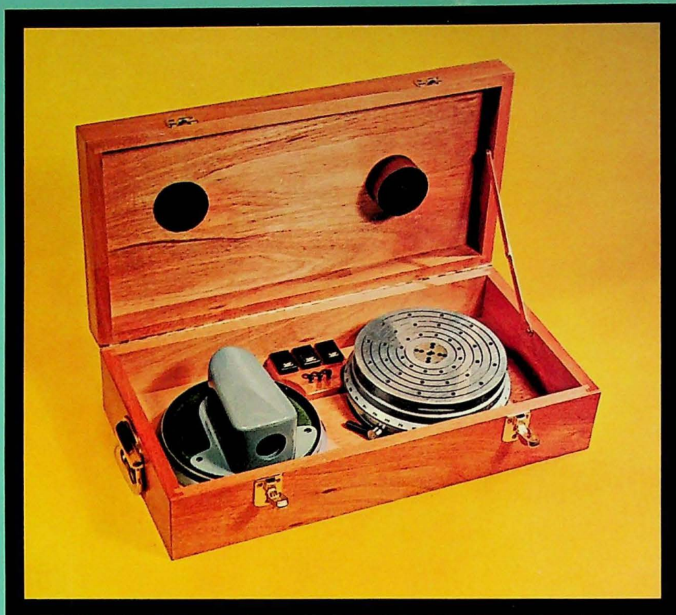
Moore 1440 Precision Index is stored in specially designed mahogany box. Convenient nesting is provided for the 1440, graduated ring, mirror housing, and clamps and screws.
