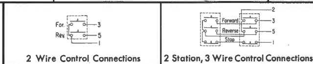
2 Wire Control Connections
