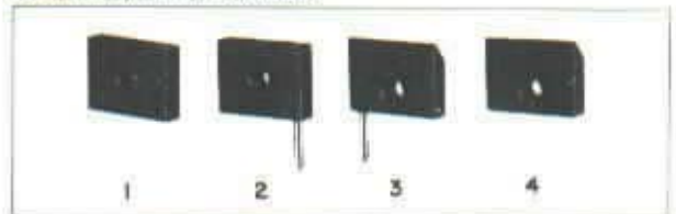
Fig. 6 Jaw set No. R-84-D. These jaws incorporate a pair of steel pins. The pins, inserted in the bottom of the lower jaws are used as guides for a template secured to the top of the work piece. These jaws are reversible. All four are drilled so the pins can be changed to the other pair when it is desired to reverse the jaws.
