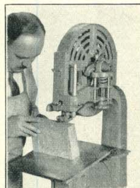
Light illuminates working area and does not shine in operators eyes.
