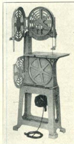
Blade is fully guarded, exposed only at working point.
