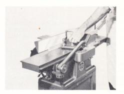
Dual Purpose Guard, pressure of thumb holds small pieces down while guard controls side pressure.
