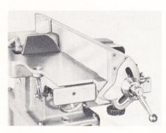
New quick action fence lock. One lever for tilt and knob under carriage for lateral adjustment. Self-indexing at  $45^{\circ}$ .
