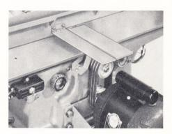
Rear knife guard keeps knives covered at all times, regardless of position of fence. Guard always in position. Does not require adjustment.
