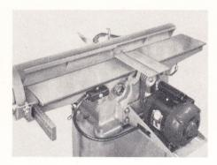
Compact self-contained unit; note conveniently located controls and lock handles, motor mounting and triple V belt.
