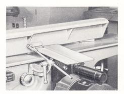
Showing new fence support, fully adjustable and assuring rigidity to fence in all positions.
