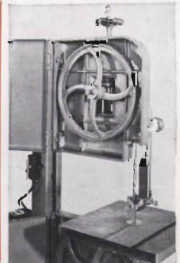
BW740 Band Saw shown mounted on IJ110 X Stand, necessary belt, pulley and motor rails are listed above.
