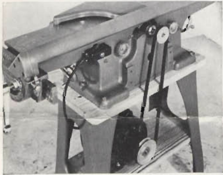
Motor may be mounted under or behind the machine. Pulleys supplied with machine give cutter-head speed of 3800 rpm. MB1 Motor Rails listed above may be used to mount the motor.
