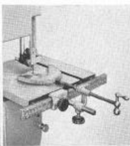
Using screw feed to cut cylindrical piece of steel.
