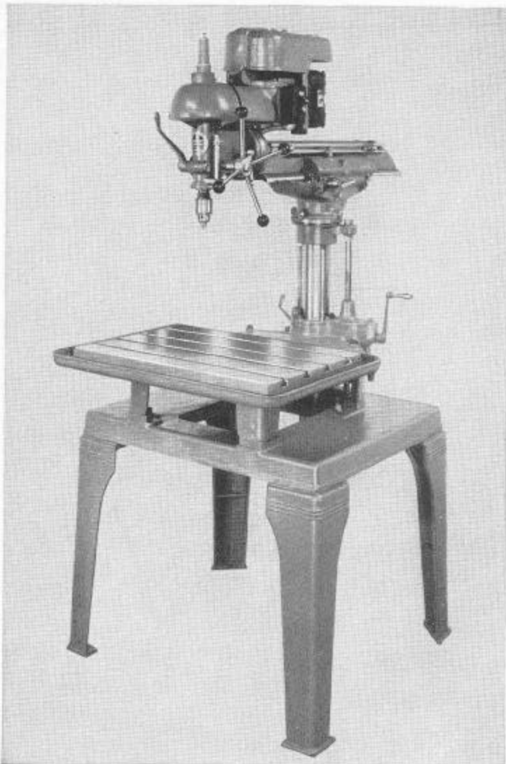
A. The drill head and motor assembly can be tilted in either direction to any angle up to 45°.
