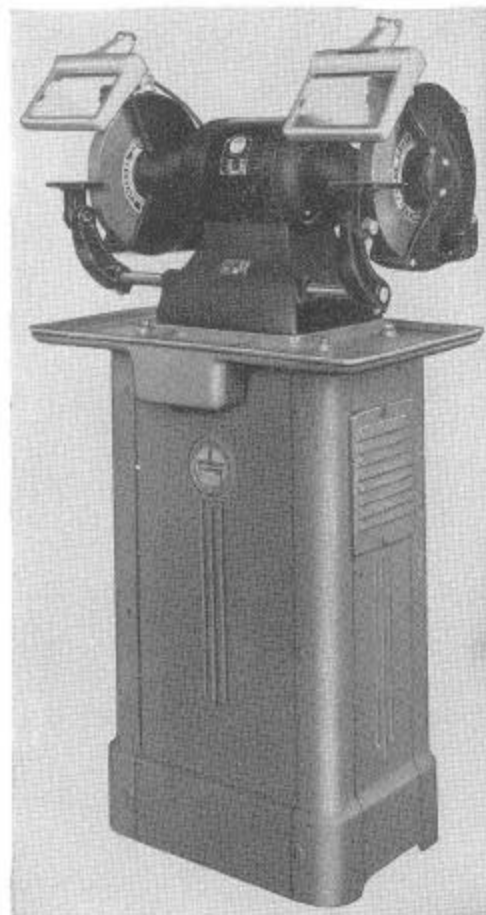
GR100 1 h.p., 1725 r.p.m., 220/440 volt, three phase Grinder as shown with 2 wheels 10" x 1" x 3/4", less Eye Shields and Base (3 phase only) GR100A Shatter-proof Eye Shields GR101 Cast Iron Base
