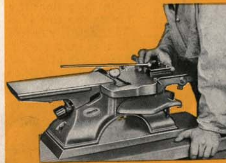
The cutter head is tested for alignment with the tables by a delicate gauge which shows variations in thousandths of an inch.
