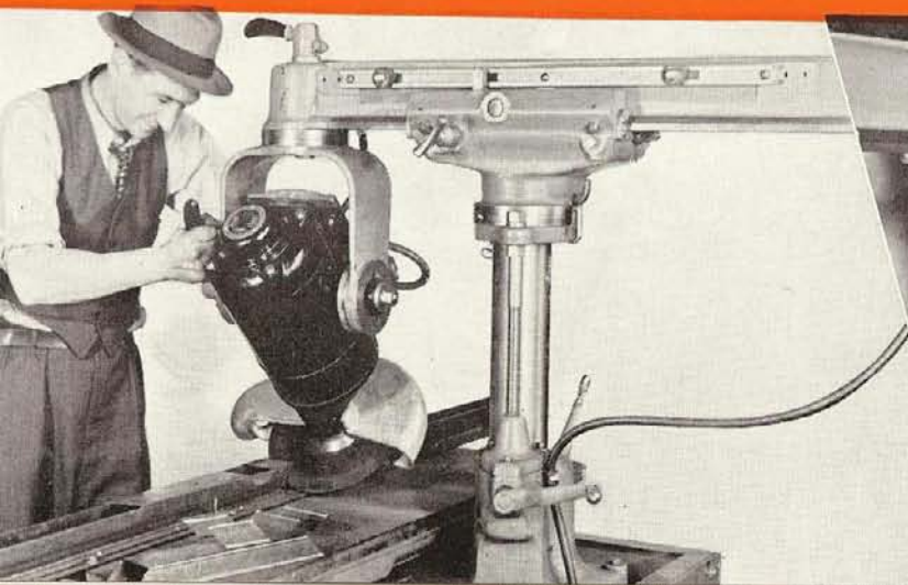
Formed steel moulding held on a special fixture is accurately cut to 45°.
