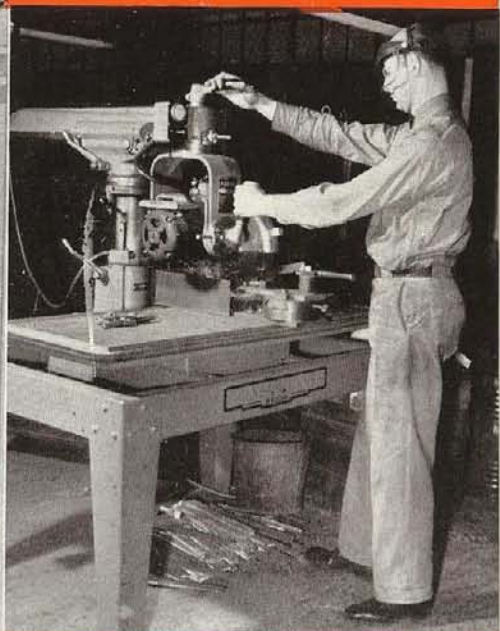
This photo shows the motor turned 180° to facilitate a special cutting operation.
