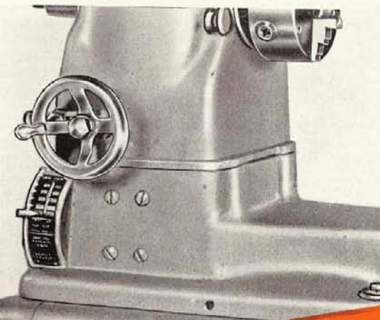
The hand wheel provides infinitely variable spindle speeds within the range specified.
