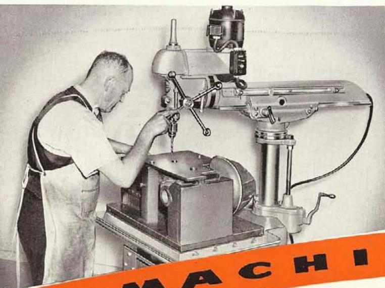
In the toolroom or on the production line the W-T Radial Drill performs drilling, tapping, routing, light profiling and other such operations with speed and accuracy.
