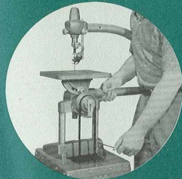
SETTING TOOL HEIGHT FOR RIGHT BELT TENSION
