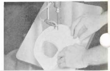
JIG SAWING AT 45 DEGREES
