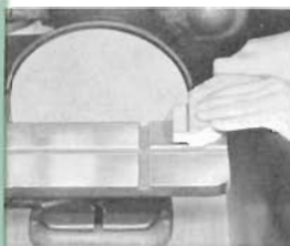
SANDING INSIDE CORNER
