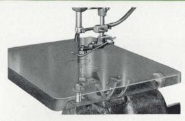
The 14" x 14" table with its full unbroken working surface on all sides of the blade can be tilted  $45^{\circ}$  to either the right or left. The two jaw chuck can be rotated  $90^{\circ}$  for working long stock from the side of the machine.
