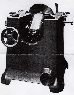
The totally enclosed, fan-cooled, dust proof motor is mounted on a frame that swings on accurately machined segment gibs... The dust outlet is cast integral with the base.
