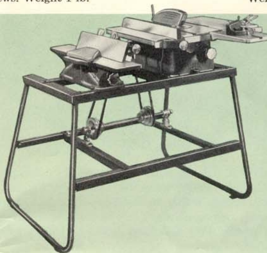
TS-99 ALL PURPOSE DUAL STAND. The Dual Stand has been designed for mounting more than one tool with one motor. The 8 inch Tilting Arbor and 4 inch Jointer, controlled with one motor, are shown as example. Stand includes Jack Shaft Y2010A, making possible mounting of other combinations of individual tools with one motor, such as band saw, sander, etc. This compact arrangement is a saving in space, and price of motors.
