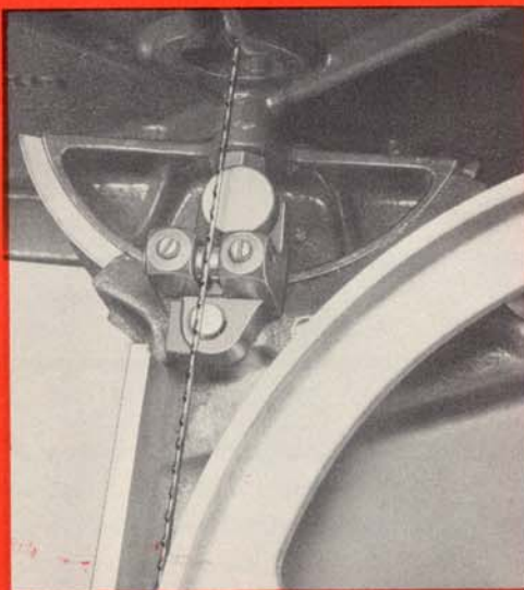
Above photo shows integral part of the SHOPMASTER Blade guides. Shows the hardened steel thrust guide as well as the brass side guides and longitudinal guides. It also incorporates exceptional trunnion construction. Upper guide same construction.
