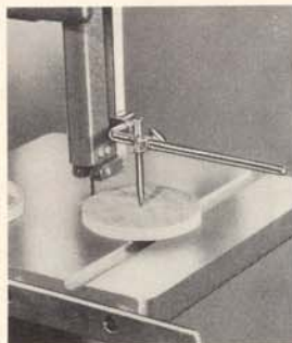
CA-210 SHOPMASTER Band Saw Circle Cutting Attachment. Will cut circles from 2" to 10".
