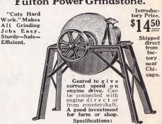
Drive Pulley—12x2½-inch face, Geared 5 to 1. Speed, 20 R. P. M. Stone—High quality; free cutting. Size, 22x4 inches. Weight, 123 pounds.
