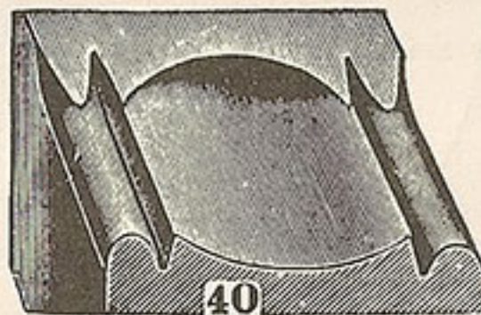
Sectional Views Showing a Few of the Cuts that can be Made with the New Former Knives, Described on Page 25
