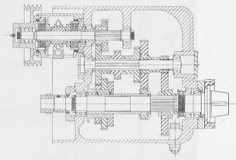
HEADSTOCK — twelve spindle speeds. All sliding gears on the initial drive shaft, intermediate shaft, and the spindle back gear, operate on multiple splines for ease of shifting, balance and maximum driving power. The double row Timken precision bearings on the spindle take all thrust close to the spindle nose providing greater accuracy and longer life. Rear spindle bearing is preloaded Duplex type assuring maximum accuracy regardless of thermal expansion of the spindle.
