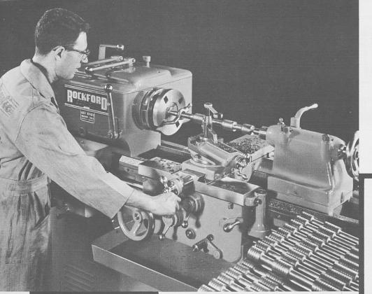
ACCESSIBILITY . . . All pick-off change gears, reverse gears, etc. as well as the main drive sheaves and vee belts are readily available for inspection by the opening of a one piece hinged metal guard at the Headstock end of the lathe. All moving parts, with the exception of the spindle nose, are well guarded to prevent injury to the operator.
