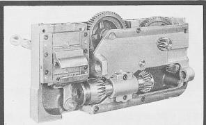
APRON (above and below)—double wall construction gives front and rear bearing support for all gear shafts.
