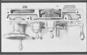
**HEADSTOCK** . . . Provides a range of twelve spindle speeds, with any speed quickly selected by means of three conveniently located gear shift levers. Gear shafts are metallurgically and mechanically designed with ample margin of load safety; all shafts are anti-friction bearing mounted. The Spindle is made from a high alloy steel forging, has a 1-9/16" hole, and is mounted on Timken zero-precision bearings. The Spindle nose has a No. 1 tapered key drive.
