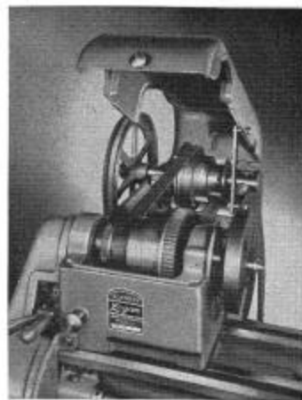
HEADSTOCK AND COUNTERSHAFT WITH GUARD RAISED
