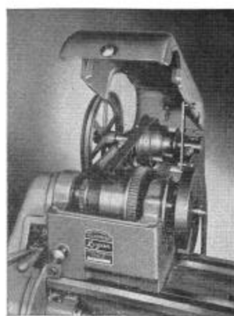
HEADSTOCK AND COUNTERSHAFT WITH GUARD RAISED
