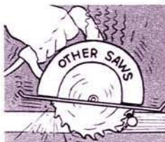
When blade on conventional saws are suddenly stopped, motor often burns out.
