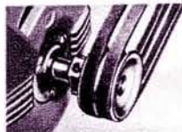
Dual belt drive delivers more HP to blade
