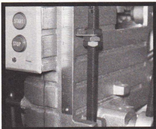
Micrometer —Type depth gauge assures depth accuracy with precision, eye-level calibrations. Easy to set, easy to see!
