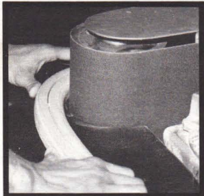
Contour sanding on the rubber covered idler drum is simple by removal of a dust hood.
