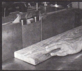
A unique felt and graphite covered roller assisted center platen provides an ideal method of jointing and sanding a straight edge during the same operation. Both cast iron faceplates are quickly adjusted and locked in position for real precision finishing.
