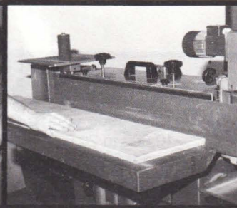
A full 33" sanding platen insures precision edges on short or long stock.
