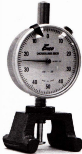
Cutter Head Gauge —Chrome plated plunger type gauge mounted on cast iron base. Designed to rest squarely on cutterhead for fast micrometer accuracy in setting knives. Part No. 2230007.
