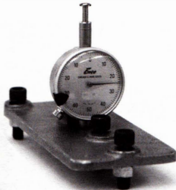
Bed and Feed Roll Gauge —Dual purpose . . . gauge mounted with swivel on cast iron base with leveling screws for simplified operation. Dial face rotates for easy zeroing. Part No. 2230002.
