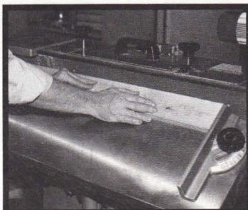
Rear table may be raised and lowered full belt width for straight edges or tilted for bevel sanding.
