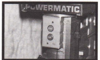
Safety Control Switch is front-mounted for operator convenience. Guarded push-button design helps prevent accidental starts.
