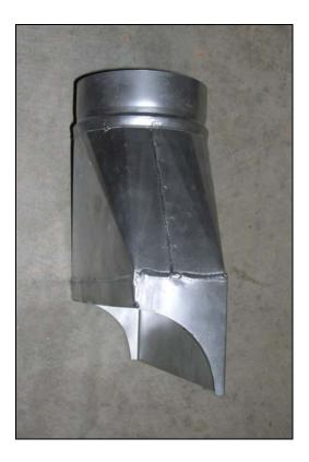
This hood has a 6" diameter outlet which can be connected to your dust collection system with an appropriate size reducer. I purchased a stock 6" x 4" reducer from the BORG to connect the hood outlet to the 4" flexible hose on my dust collector.
