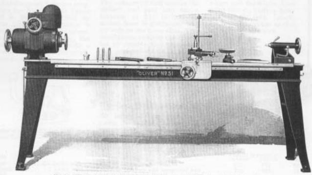
No. 51 "Oliver" Adjustable Speed Motor Head Laths with Eight-Foot Bed Fitted with Carriage, Compound Swivel Rest and Set-Over Tailstock-s Real Good Lathe.
