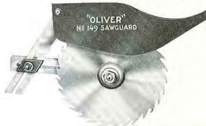
Thousands of these guards are in daily use, giving satisfaction. A clamping plate, steel spreader and hardwood duck make up this guard. The spreader or "splitter" prevents pinching and throwing lumber back.
