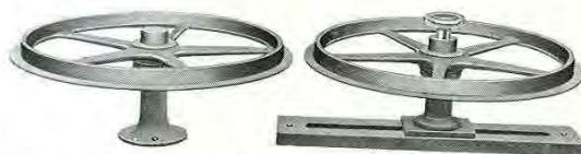
mounted for use one is stationary and the other has 12" adjustment. They are fine to use in supporting a band saw blade when filing or setting it.
