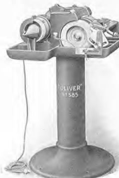
Left side view—Note emery cone, leather Stropping wheel as well as two oilstone wheels and tool holder
