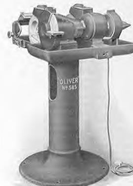
Right side view—Note emery wheel with tool rest as well as two oilstone wheels and tool holder
