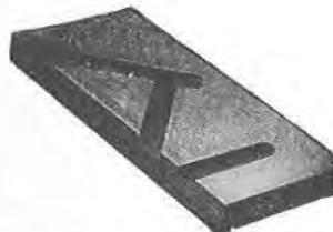
No. 4. Section of Stair Stringer grooved by  $\frac{7}{8}$ " routing cutter.
