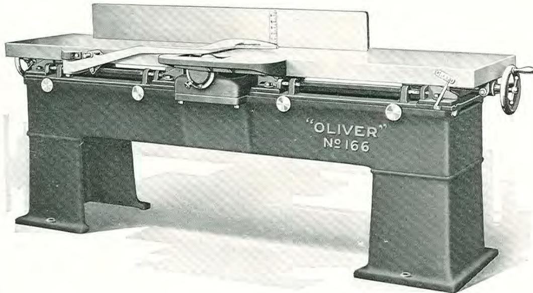
Front View Showing "Oliver" Aluminum Automatic Guard Mounted in Place
