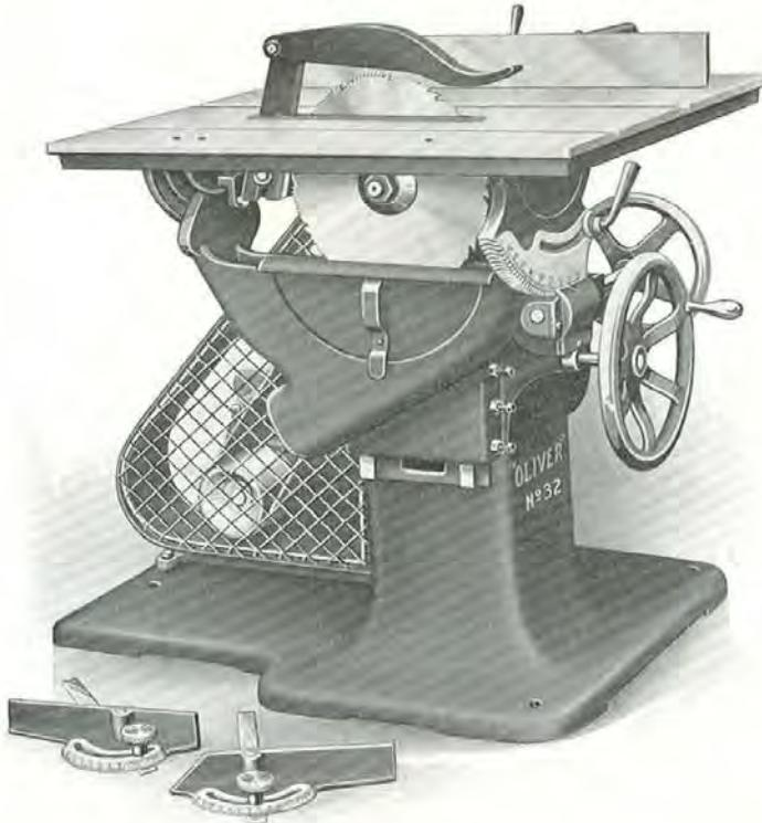
**Motor Driven as Shown or Belt Driven with Self-Contained Countershaft**
