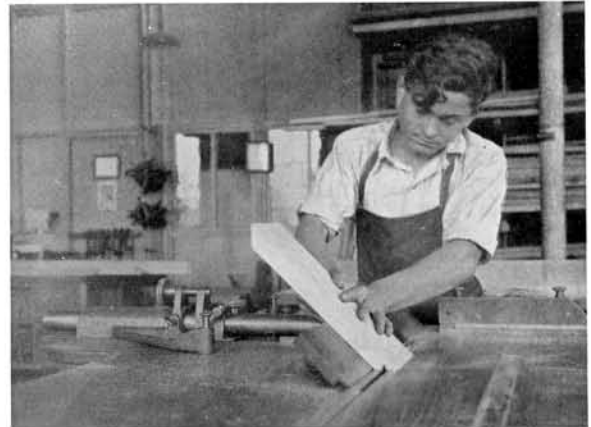
FIG. 43 Grooving—making splined miter joint with dado or grooving saw—fence at an angle
