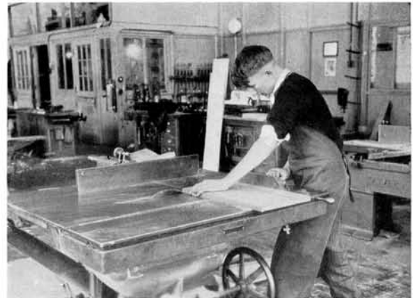
FIG. 27 Crosscutting—stop rod on cut-off gauge adjusted for length to square second end
