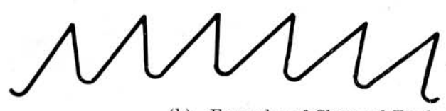
(b) Examples of Shape of Tooth and Gullet on Circular Crosscut Saws
