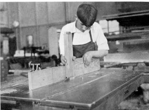
FIG. 37 Cutting tenons—cheek cut made with aid of push stick, forward end of which is cut to proper angle—stock held in correct position
