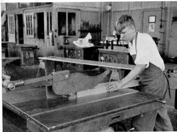
FIG. 20 Simple ripping—ripping stock to width
