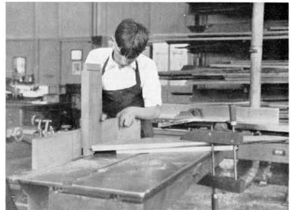
FIG. 38 Cutting tenons—cheek cut with aid of push stick and feather board which holds stock against fence and serves as guard over the saw
