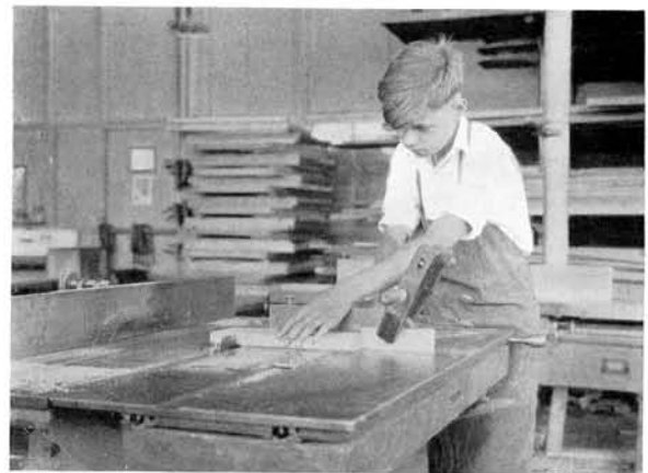
FIG. 28 Simple crosscutting—using block of wood clamped to gauge for stop
