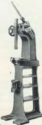
No. 2 5 Tons on Pedestal
