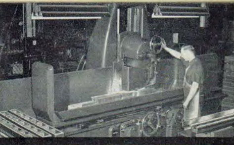
Precision-Grinding Lathe Bed Ways
