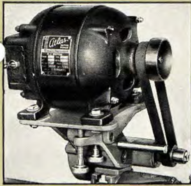
View of 10-450 heavy-duty lathe grinder with belt guard removed, showing two-step pulleys, built-in switch, and belt-tensioning screws.
