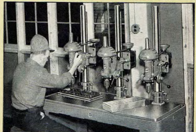
This new Atlas W-83 three spindle drilling machine has reduced costs by 40%. Each control plate requires over 100 holes (3 sizes).
