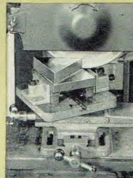
Magnetic chuck of grinder holds W68 vise while sides of triangular die are finish-ground.
