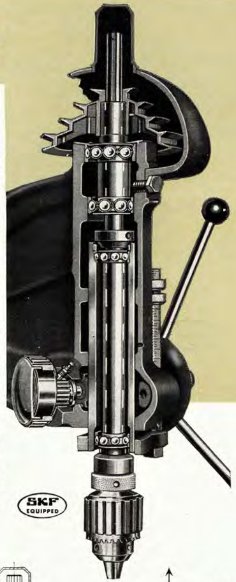
Above: Spindle-Head Bearing Construction of Nos. 63 and 73 Drill Presses from left side. Notice four large deep-grooved SKF ball bearings, floating-drive design, splined spindle and drive pulley, precision-bored quill guides and drive-bearing housings. Dotted line indicates drill press spindle.
