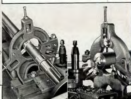
(Right) Steady rest supporting axle for turning and shaft for facing end.
