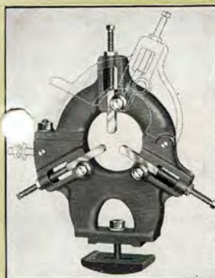
(Right) Steady rest supporting axle for turning and shaft for facing end.
