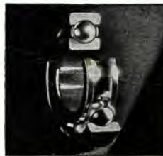
Cross-section view of large deep-grooved SKF ball bearing used in Nos. 63 and 73 spindle-head bearing design. Two of these bearings support floating spindle drive unit in head—two more float the spindle free from the quill.
