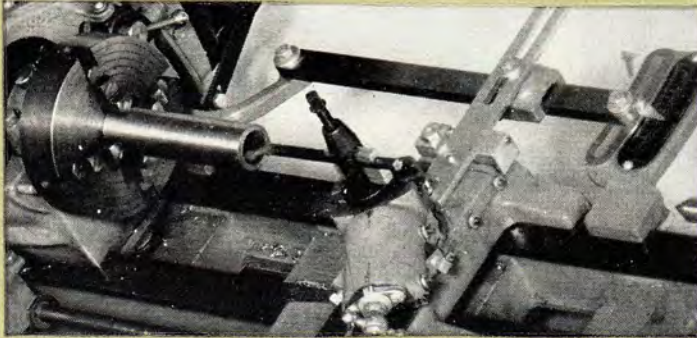
The taper attachment makes boring an easy job. Here the No. 760 attachment is boring a tapered socket.
