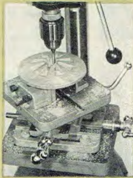
The W68 vise simplifies many jobs in the pattern shop. Above, routing angular slots.
