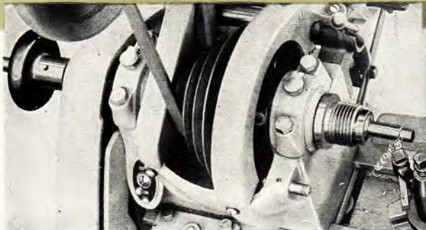
No. 750 Draw-in Collet Chuck Attachment in operation—collet is controlled by handwheel at left.
