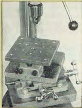
A typical spacing job for the W68 vise—drilling holes at 60° intervals around center of drill jig.
