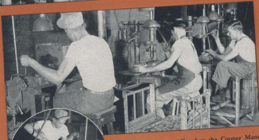
Unique combination of 4 Atlas drill press heads set up to drill 4 holes simultaneously at the Pacific Enamel Works, Richmond, California. Air-operated fixtures position the piece, then after a timed interval air cylinders advance the drills.
