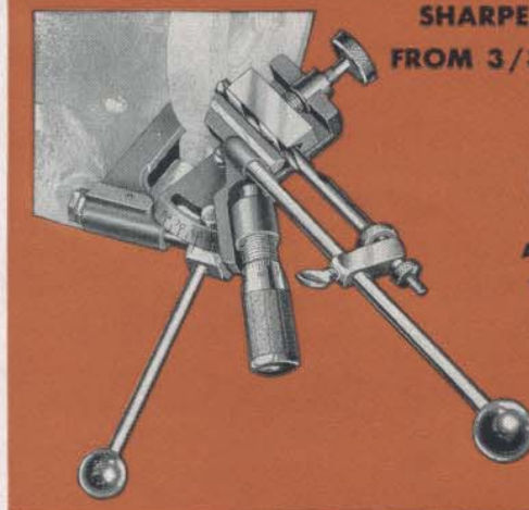
Here is vise table alone (No. W68-2A) replacing compound rest on Atlas 10" lathe, to hold long piece for boring.
