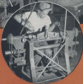
Output went up 300% when the Cooper Manufacturing Co., Marshalltown, Iowa, installed this Atlas drill press "production line." Two horizontally mounted heads enable operator to see work clearly and simultaneously countersink both ends of bar. Jigged part then goes to next operator for 7 holes, and to end of line for two more holes and tapping.
