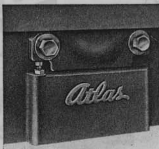
Fig. 9 Two bearing hanger screws and an adjusting screw are used to accurately position cutterhead and blades in relation to rear table.
