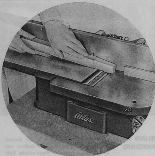
Fig. 19 Cutting a short taper.
