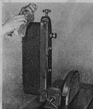
Fig. 2. Contour sanding with the Belt Sander in vertical position and belt guard removed.
