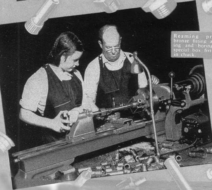
Turning special stud at Progressive Tool Works. One of a large battery of Atlas lathes on continuous production.
