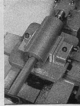
Vise table alone (No. W68-2A) holding long piece for boring in Atlas 10" lathe.
