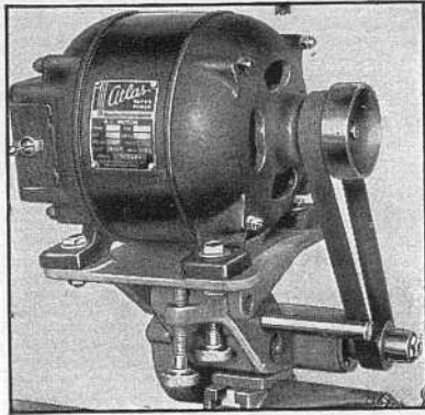
View of 10-450 heavy-duty grinder with belt guard removed, showing two-step pulleys, built-in switch, and belt-tensioning screws.
