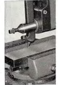
HORIZONTAL CUTS (Work in Vise)
