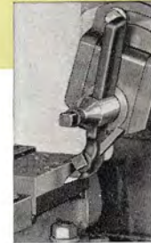
VERTICAL CUTS (Work in Vise)
