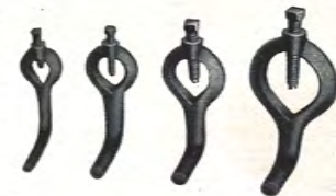
FIG. 80 Lathe dogs for driving work up to 1½ inches in diameter.
