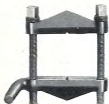
FIG. 83B Holding rectangular work in the clamp-type dog.
