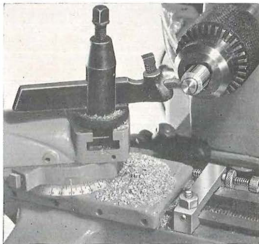
FIG. 221 Another view of the same repeat operation shown in Figure 195. This angle shows how the cross slide stop gauges the depth of the cut. Note carriage stop in background.
