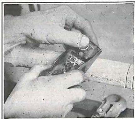
FIG. 302. Smoothing down work with the small block plane.
