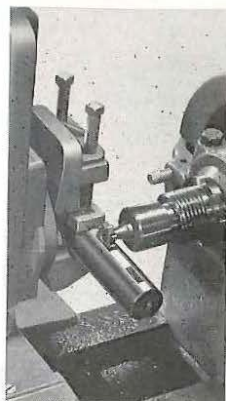
FIG. 226 Milling a Woodruff Keyway.
