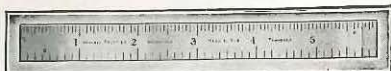
FIG. 270. Flexible steel rule graduated on two edges. Handy for measuring tailstock setover.
