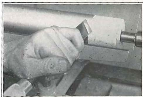
FIG. 298 Taking a finish cut with the large skew chisel.
