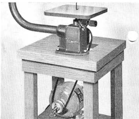
2 Motor mounted on shelf beneath jig saw.
