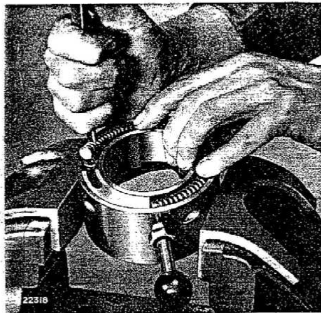
4. Replace the pads in the ends of the opening spring and, using a screwdriver, place the spring in the internal scroll.
