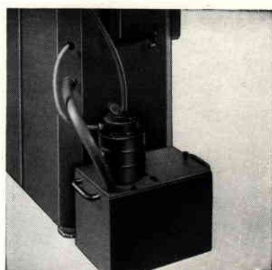
Coolant tank and submersion pump mounted externally at side of Cabinet showing wiring, delivery and return pipes.
