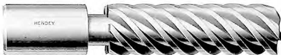
Screw with six starts and four inch lead.*
