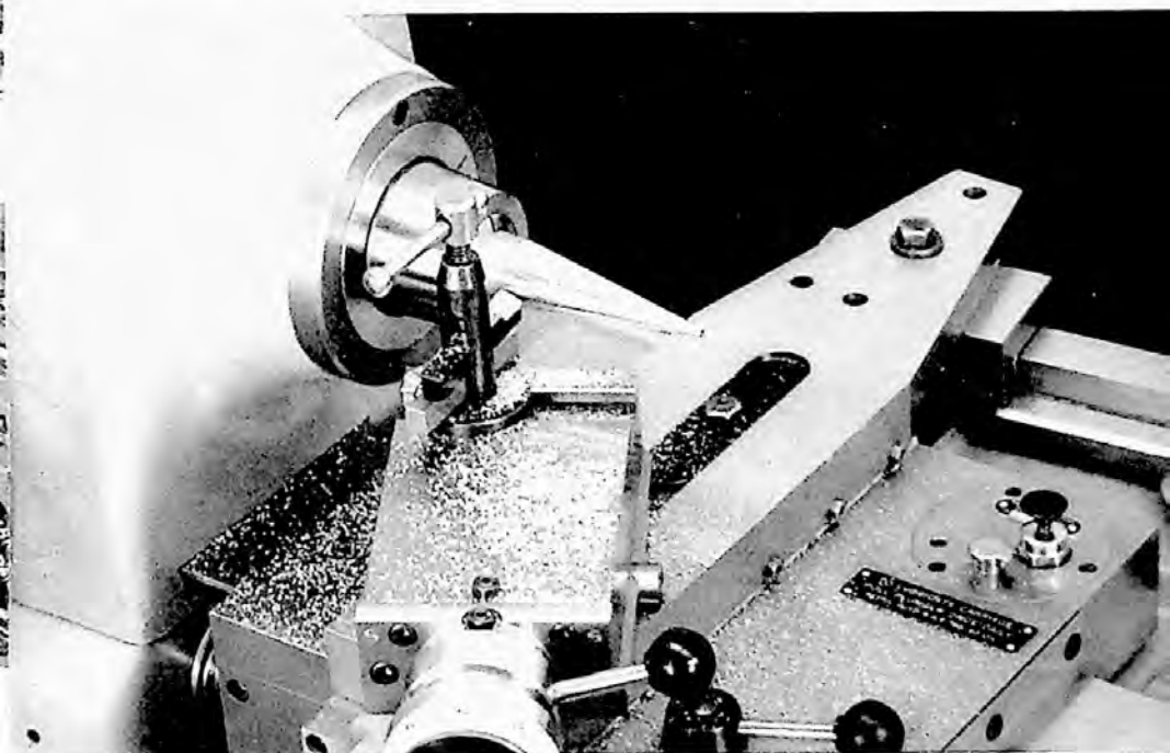
Precision taper turning is easy when done on the Hardinge HLV Lathe equipped with a taper turning attachment.
