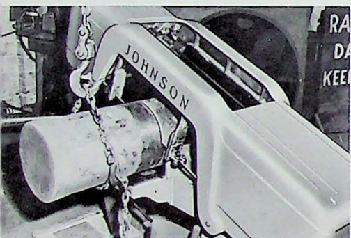
Although not recommended for continuous daily procedure, this Johnson "J" rapidly and accurately slices through a 12" steel ingot — another example as to why Johnson Saws are preferred for performance — everywhere!
