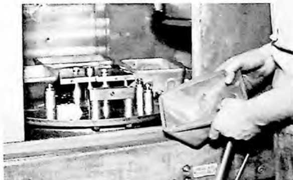
Box Castings — By putting fixed locating plates and a few adjustable bolts for positioning the work atop a mounting plate, four castings can be ground at once. The plate covers the whole chuck surface. A little ingenuity will produce such a chuck for almost any part.
