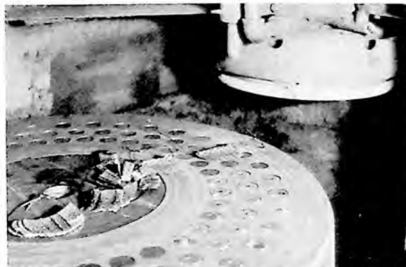
Difficult Shapes — Small pieces that do not block well can be nested in holes in a non-magnetic masking plate located to position workpieces over the strongest parts of the chuck. Here, small thin gears, like those strung on wires at the middle, are nested.
