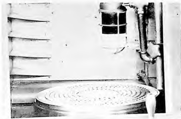
Blocking Small Pieces — To counteract the tendency of the grinding action of the wheel to move parts on the chuck, blocking rings may be used. Here two rings (supplied with the machine) block the small disks and hold them in contact with each other.
