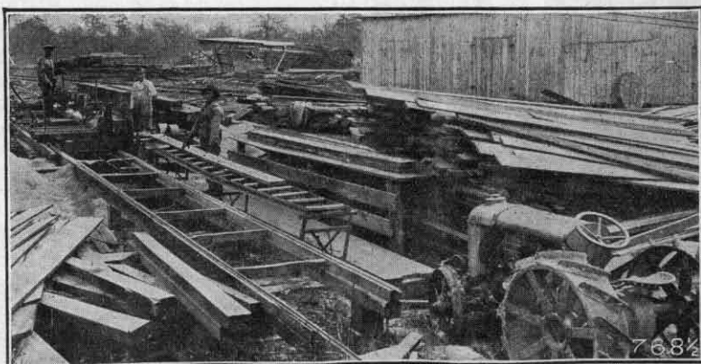
No. 2 Saw Mill and Farm Tractor in Virginia 1,025 ft. of 1-inch boards in one hour.
