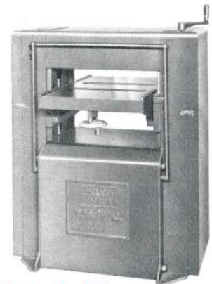
Max 16" x 6" Planer Model MF-16 3 HP Motor . . . Shipping Weight 1100 lbs.
