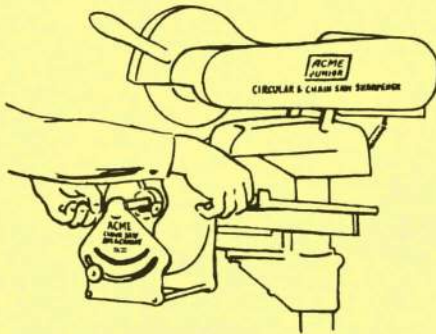
1. Place the attachment on front bar of the sharpener.
