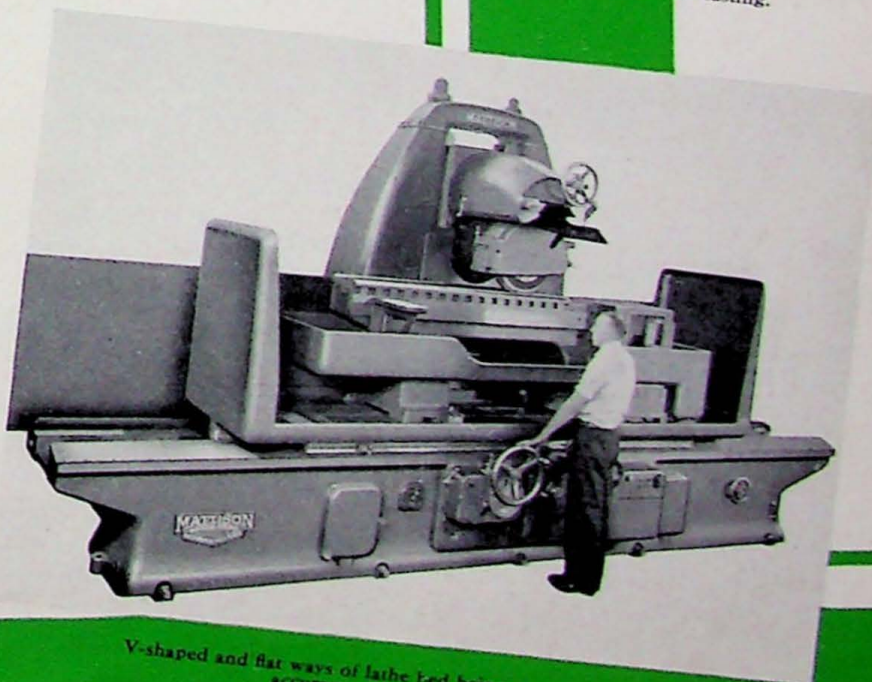
Mattison Grinder holds close limits on 3-4" high 3000 pound base casting.
