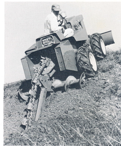
60.5-hp V-461D on trencher-blader
