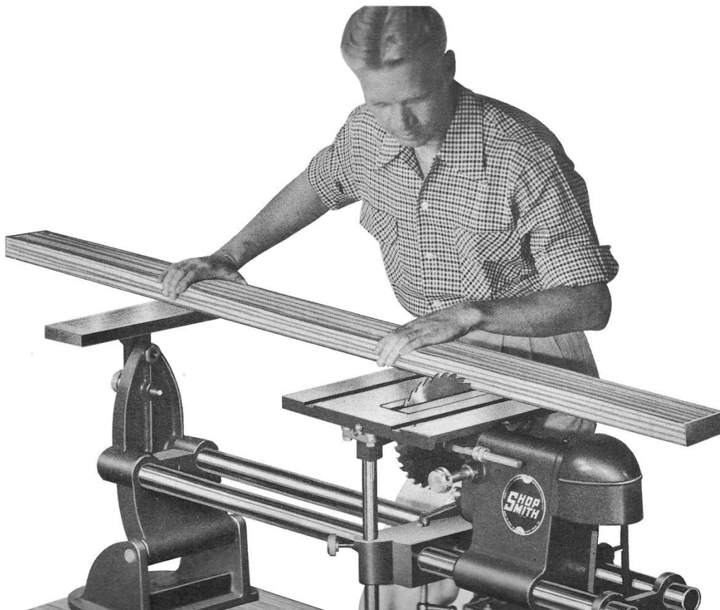
FIG. 14 Crosscutting long board using extension table for support.
