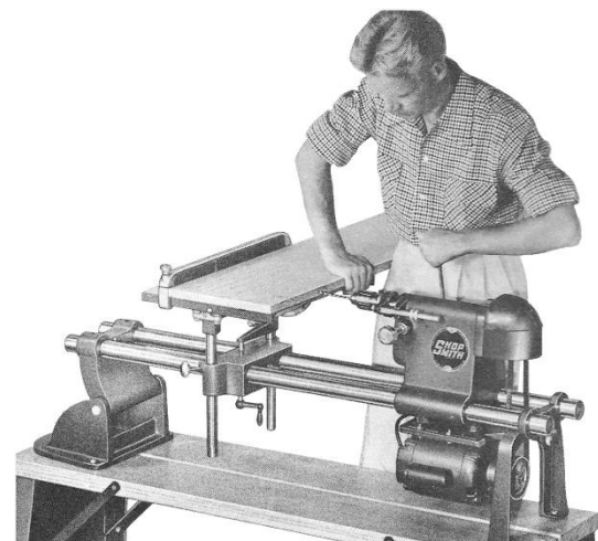
FIG. 18 Drilling for dowelling in horizontal position using rip fence as back-stop.
