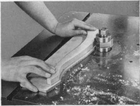
Shaping with slotted collars. (Universal guard removed to show detail.)
