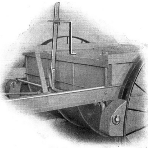
Method of attaching Brake on DX, BX, EX and CX.
