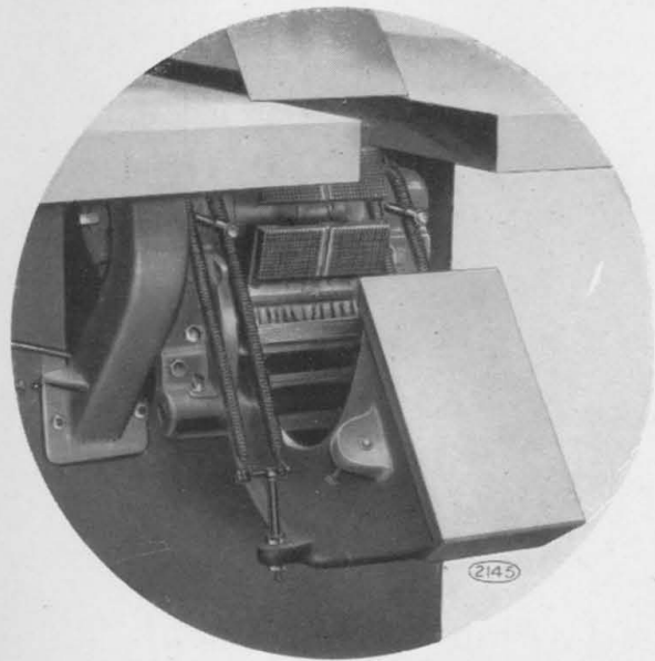
Section of End Table lowered, giving access to Chain and Brush
