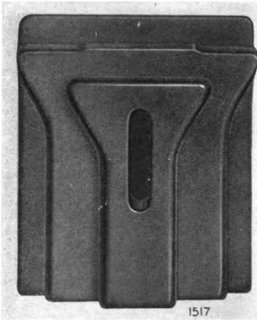
Former Block to Aid in Correct Forging
