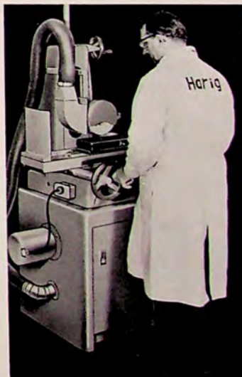
Built in dust collector system on Hand Feed Model. (Exterior collectors on Automatic or Hydraulic Longitudinal Feed Models.)
