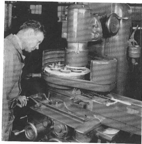
Circular grinding attachment complete with rotary magnetic chuck can be provided as shown.
